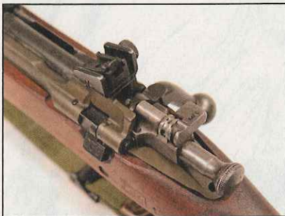
Like the Model 1903, the O3A3's safety was located on the bolt. When the catch is to the left, the gun is ready to fire, and to the right, on safe.
