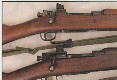
Slight manufacturing differences occurred between manufacturers, such as the more rounded trigger-guard seen on the Remingtons (top) as opposed to the slightly flatter ones on Smith-Coronas.
