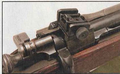
The rear sight of the O3A3 was placed at the rear of the receiver and was considerably simpler than the ladder-style of the earlier m1903. many parts were stamped.
